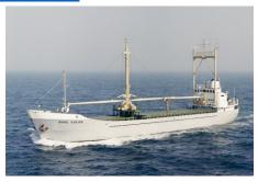
IDNo: 6620888 - Year: 1966 - Name: CITY OF ROTTERDAM - Type: Cargo ship - Launch Date: 3.9.66 - Flag: DEU - Date of completion: 21.9.66 - GRT: 499 - DWT: 11170 - Yard No: 590 - Length overall: 68.4 - LPP: 62.1 - Country of build: DEU - Beam: 10.5 - Builder: Sietas of Neuenfelde.
